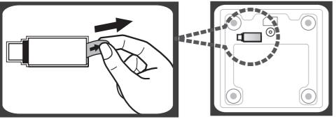
**EN** **BATTERY** 3xAAA battery. Please remove the isolation sheet from the battery contact before use.
